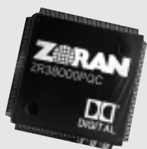
Zoran introduces first single-chip processor capable of Dolby AC-3 digital audio coding and decoding. First used in second-generation DA20 Dolby Digital film sound adapter.
